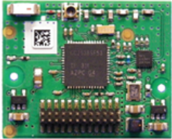
ZigBee® Pro Wireless Card ZVRCZPWC2
